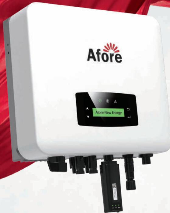
The Afore HNS Series Single-phase inverters are designed for residential PV system applications, rating from 3kW to 6kW. All models have unibody housings with aluminum structure which is anodized, increasing durability and effectively prevents corrosion. Equipped with external inductors, the unibody housings can ensure efficient heat dissipation, which significantly improves the reliability and extends the life of the inverters.
